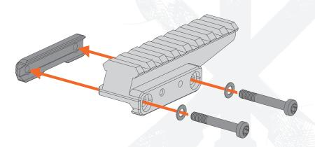
1 Secure screws using a T25 bit driver. Lightly snug all screws before applying final torque to any. DO NOT EXCEED 35 IN-LBS.
