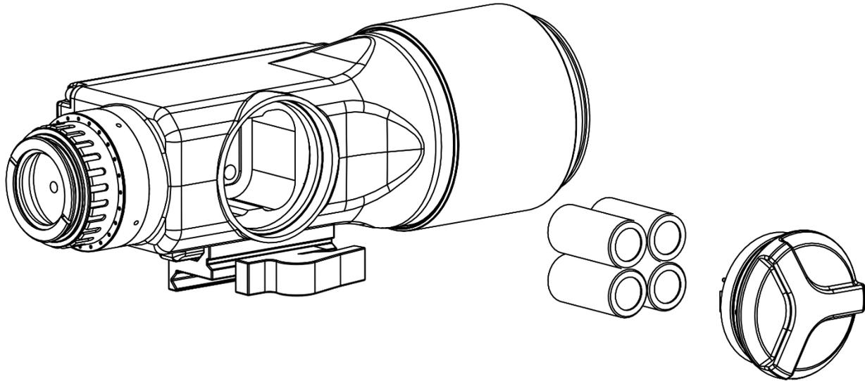
**Figure 3. HALO-LR With Removed Battery Compartment**
