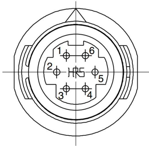
**Figure 10. HALO-LR Electrical Connector**
